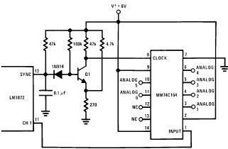
b) Six Channel Auxiliary Decoder
