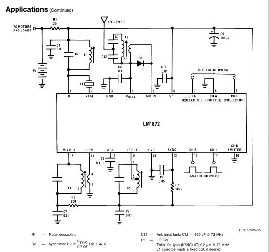
R3 Mixer decoupling C1 - LO bypass; optional C2 LO tank: C2 = 22 pF @ 72 MHz СЗ Ant. input tank; C3 = 24 pF @ 72 MHz C4 V<sub>BIAS</sub> bypass - Motor decoupling — Sync timer; C6 =  $\frac{\text{t'}_{\text{SYNC}}}{0.7 \text{ R2}}$ , C6  $\leq$  0.5  $\mu\text{F}$ C6 — Mixer decouple; 0.01  $\mu$ F  $\leq$  C7  $\leq$  0.1  $\mu$ F C8 — AGC C9 IF bypass; optional
