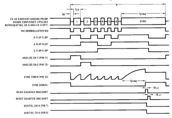
FIGURE 2. RX Timing Waveforms
